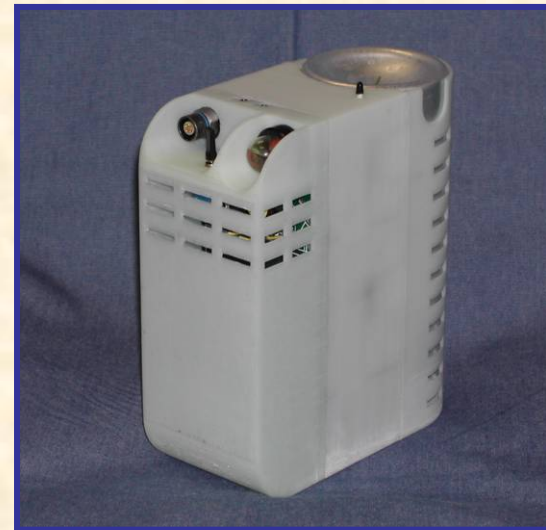
20 W Average (40 W Peak) Fuel Cell/Battery Hybrid Power Supply
