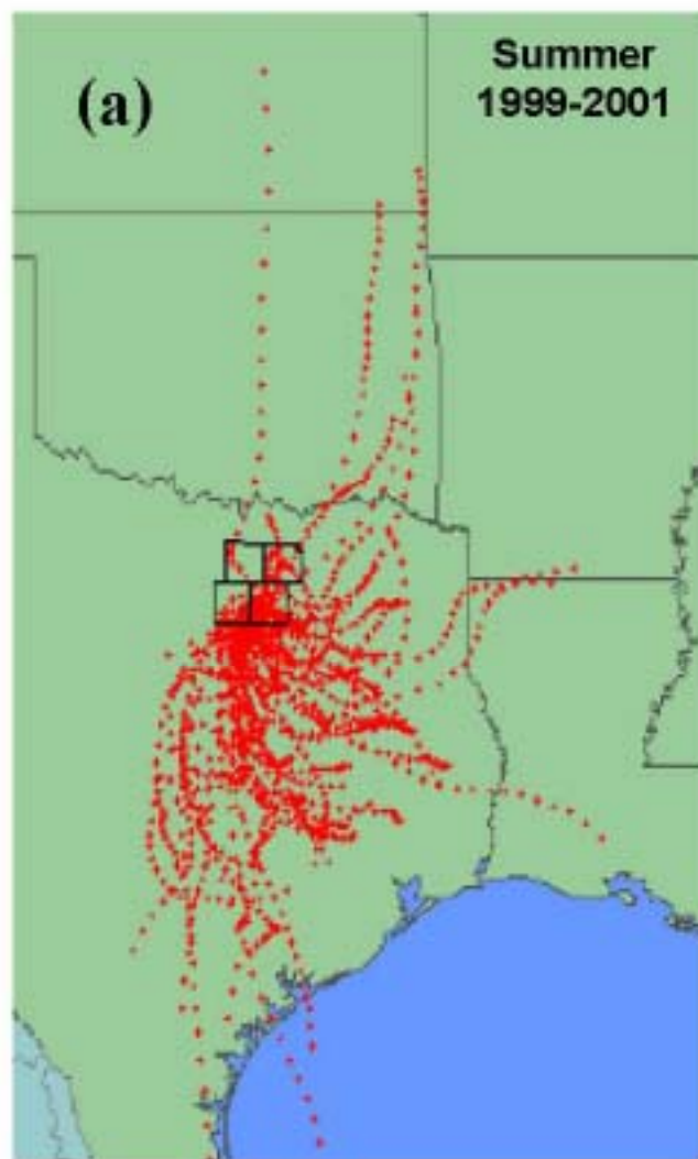
Figure 2. (a) A map of E. Texas and surrounding states showing a climatology of 24-hour back-trajectories from the four-county DFW ozone non-attainment area on high-ozone days during summers 1999-2001, and (b) a map of E. Texas showing major NO x sources. In (b), the NETPS study area of radius 250 km from Dallas is highlighted and delineated into three zones A, B, C. The impact on DFW ozone of NO x sources in these zones will be the principal goal of NETPS (adapted from Breitenbach, 2003).
