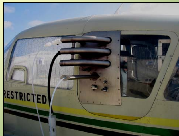
Left: Standard additions system (NO, NO 2 , SO 2 , CO & propene)
