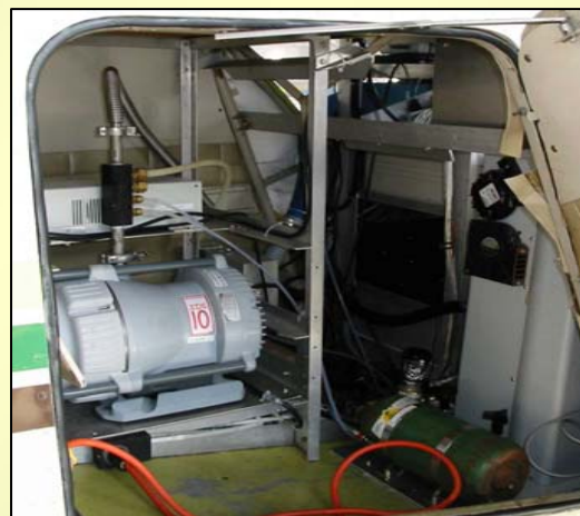
Right: Common vacuum pump for CO, NO 2 , and NO y
