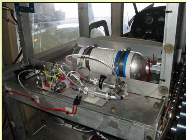
Left: Standard additions system (NO, NO 2 , SO 2 , CO & propene)
