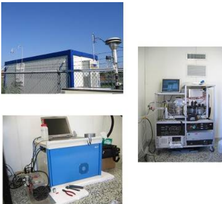
Figure 5. The instruments at the Aldine site: (top left) the trailer, (bottom left), PTR-MS, and (right) AMS.
