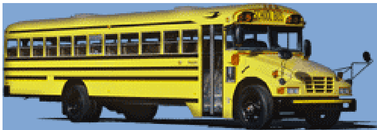
Figure 2. Illustration of the school bus type used in the current study (source: Roberts, 2006). All buses have a gross vehicle weight rating (GVWR) of more than 10,000 lbs (Type C).
