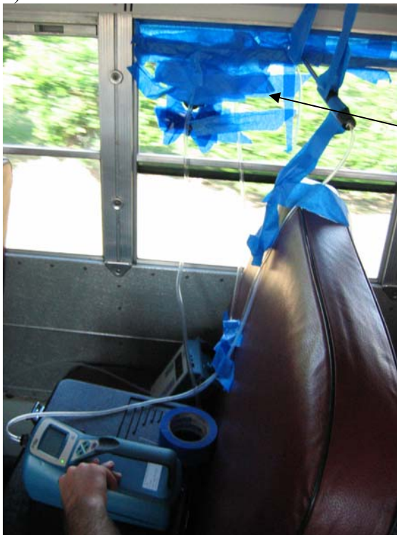
Figure 4. Instrument configuration on-board the school buses.
