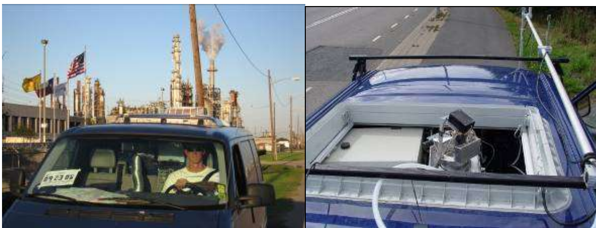
Figure 1 On the left the SOF vehicle is shown while measuring emissions from crude oil tanks not seen in the picture. The solar-tracker shown on the right transmits the solar light into the infrared spectrometer independent of the vehicle's position.
