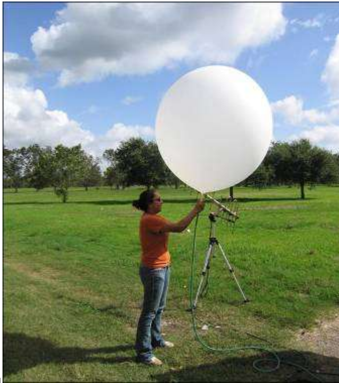
Figure 16. A GPS balloon sounding conducted within the project.
