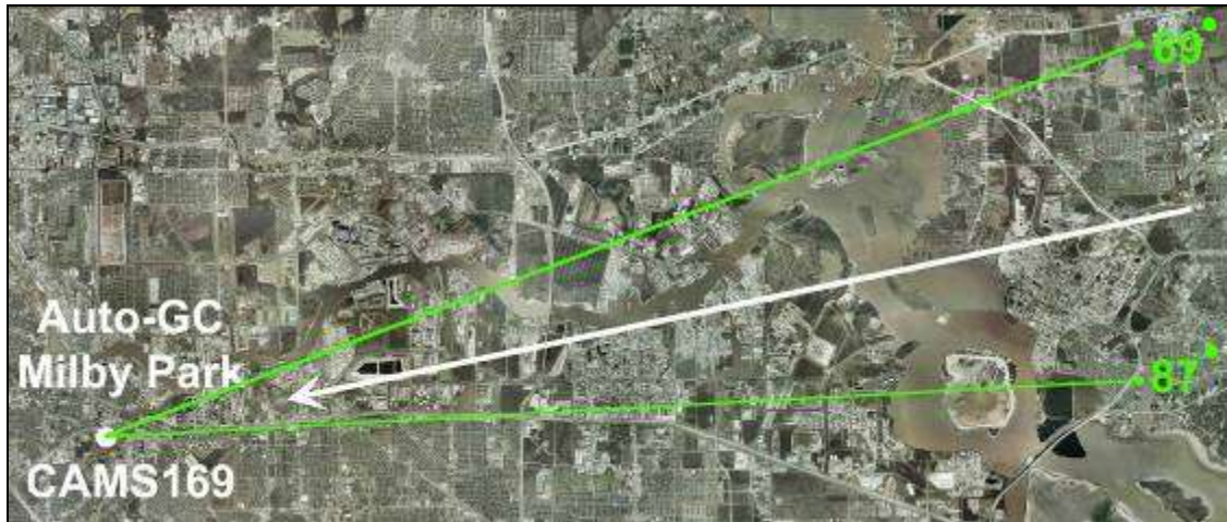
Figure 14. Location of the TCEQ auto-GC-station CAMS-169 at Milby Park in the south-western corner of the HSC area (29.706111°N, 95.261111°W). Auto-GC-data from the wind sector 69°-87° during September 2006 was used for plume speciation into 36 different compounds. (Aerial photo from Google Earth Pro).
