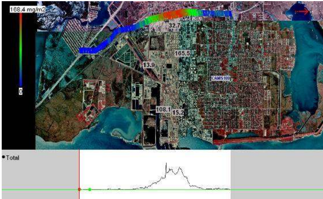
Figure 27. SOF alkane channel measurement west of Texas City on 20 September 2007, 1:42 pm. Wind from the east ( 81^\circ , 4.8 \text{ ms}^{-1} ), emission corresponding to 2905 kg/h of alkanes. Reported emissions in bold black on grey background ( \text{kg h}^{-1} ). Ground wind station CAMS100 location shown.
