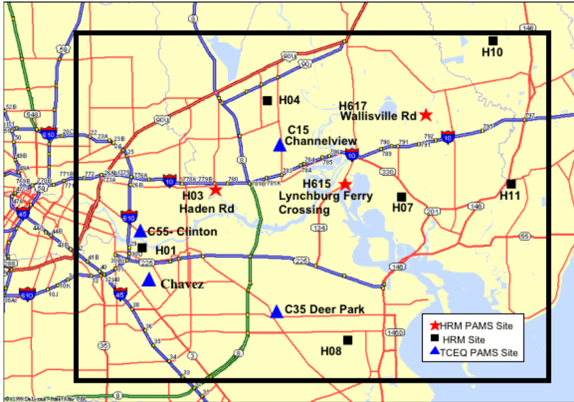
Figure 2-2. Seven-site auto-GC (“PAMS”) monitoring network used in the 2004 EMRS Houston Ship Channel pilot study (note that HRM sites indicated by black squares are not part of the auto-GC network). Source: TCEQ.
