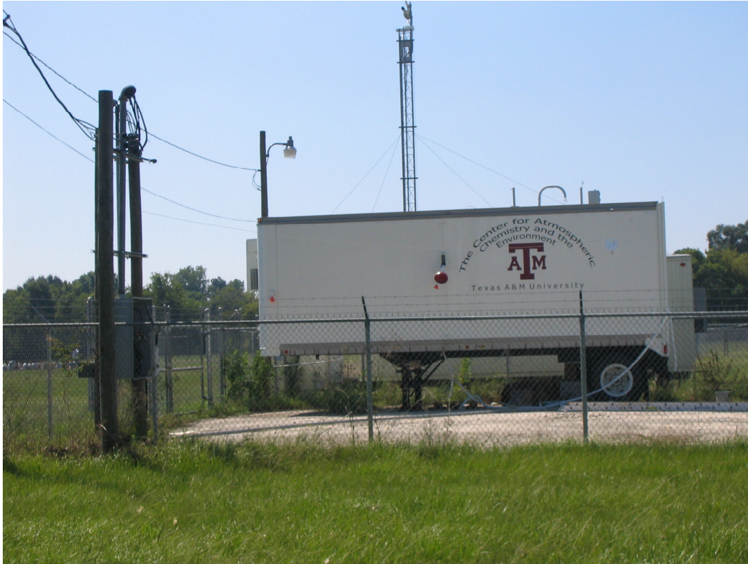
Figure 9. The outside of the trailer featuring the inlet for the ID-CIMS instrument. The inlet is a red conical device located in the center of the sidewall of the trailer.
