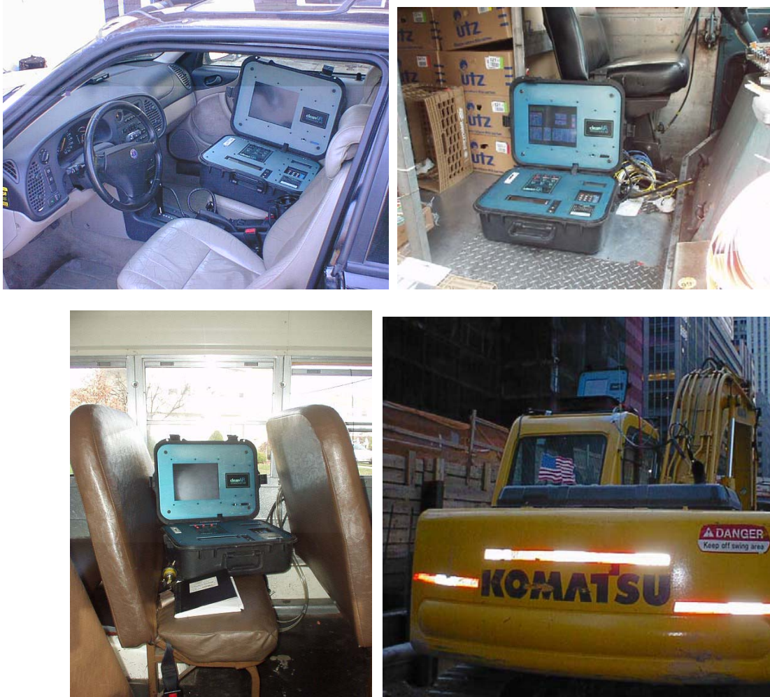
Figure 3. Examples of OEM -2100 installation locations.
